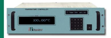
Calibration of a CES100 Series source is a quick and easy procedure using the front panel keypad and is traceable to the National Institute of Standards and Technology (NIST). The calibration procedure may be easily automated using EOI's Calsof99 calibration software, a Model LT100 thermometer and a computer with a GPIB interface. The recommended calibration cycle for the CES100 Series is six months.
